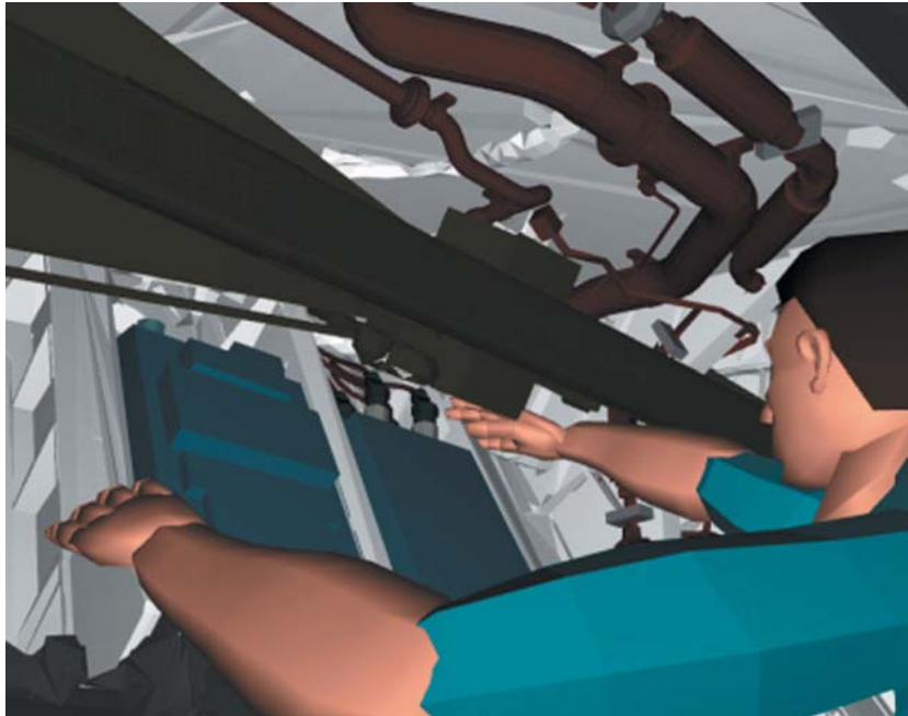
Figure 2. Jack reaching for the connectors on top of the power supply.
